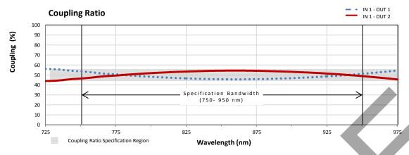
Coupling ratio (%) is the ratio of the optical power from each output port to the sum of the total power of both output ports as a function of wavelength.
