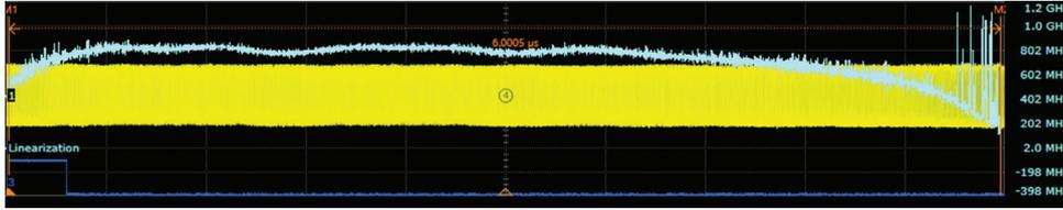
Figure 3: Scope Trace and Instantaneous k-Clock Frequency during One Sweep of 6  $\mu$ s. (This system does not pass QC due to the spikes at the end of the sweep range.)
