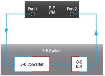
$\rm EE\_S_{21}$  is the combined through responses of the E-O Converter, EO\_S $_{21}$  and the O-E DUT, OE\_S $_{21}$  .
