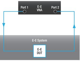
EE\_S<sub>21</sub> is the through response of the E-E DUT.
