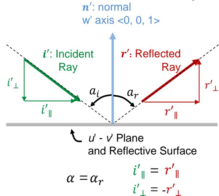
**Figure 9.** Reflection is performed using local coordinates, which involves reflecting the incident ray across the normal to the  $u$ - $v$  plane.
