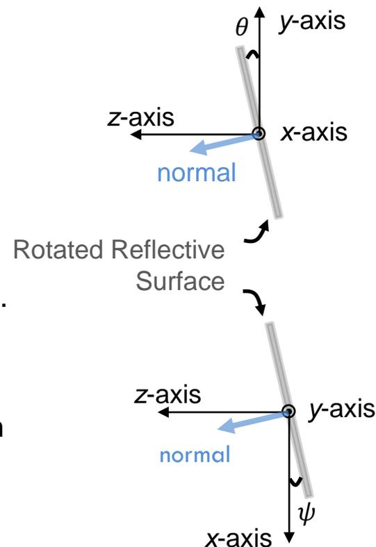
**Figure 6.** Rotation angles with respect to the x- and y-axis ( $\theta$  and  $\psi$ , respectively) are measured counterclockwise.
