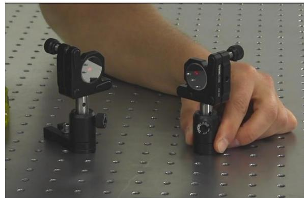
**Figure 1.** The beam path reflected by these two mirrors depends on their orientations with respect to one another.
