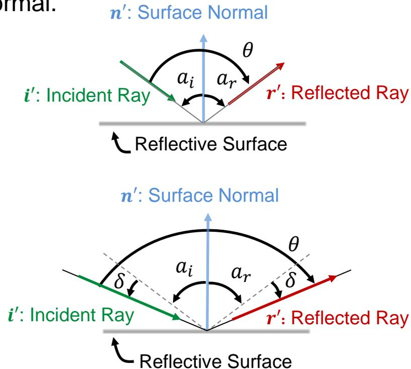
**Figure 2.** Incident and reflected ray angles with the surface normal are equal.
