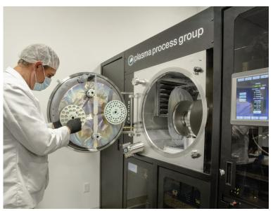
Ion Beam Sputtering (IBS) Chamber for Ultrafast Optics at Thorlabs' Headquarters in Newton, N.I.
