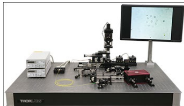
Figure 8: An optical tweezers system incorporating an EXULUS-HD1 SLM.
