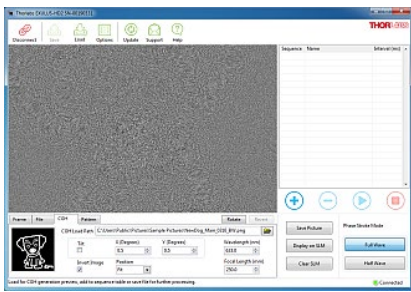
CGH Tab: Convert a user-defined image into a holographic pattern. For more details, please see the App Note tab.
