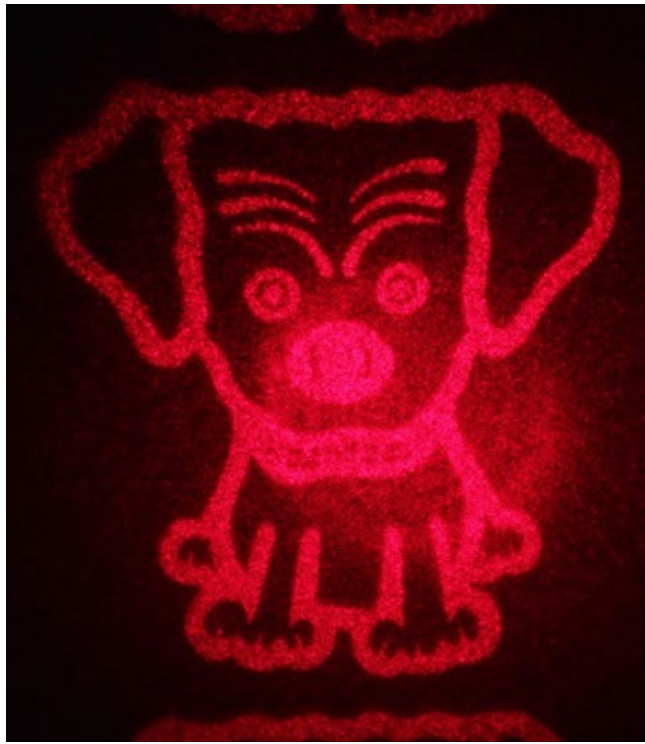
Figure 7: CGH projection of the CGH pattern shown in Figure 5 and the setup shown in Figure 6.
