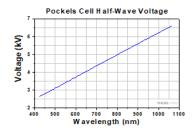
We do not recommend applying a voltage greater than 6 kV. If half-wave retardance is desired at 950 nm and above, we recommend setting the Pockels cell to act as a quarter-wave plate in a double-pass beam geometry.
