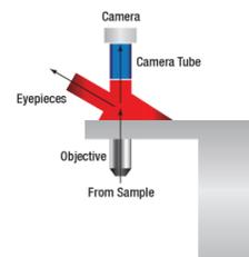
When viewing an image with a camera, the system magnification is the product of the objective and camera tube magnifications. When viewing an image with trinoculars, the system magnification is the product of the objective and eyepiece magnifications.
