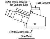
Click for Details Drawing of WFA4002 Trinoculars
