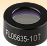
FL05635-10 Ø1/2" Filter CWL = 635 nm, FWHM = 10 nm
