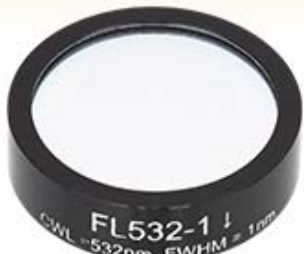
FL532-1 Ø1" Filter CLW = 532 nm, FWHM = 1 nm
