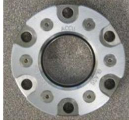
Place the screws in the face plate holes and use the 2 mm hex key to turn each screw ~1.5 turns so that they are flush with the face plate but not tight.
