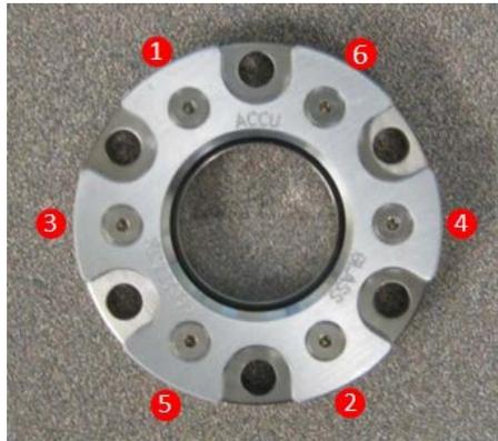
Use a torque driver set to 30 in-oz to screw in all six setscrews. Refer to the sequence shown in the pattern above for the correct order in which the screws should be torqued. Please note that over-torquing the screws will risk damaging the window. While the viewports for Ø1" windows only have 4 screws, use the same sequence for tightening the screws.
