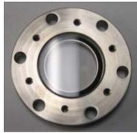
Install the o-ring in the seat, and place the window on top of the o-ring (left image). Place the face plate on top of the window (right image).
