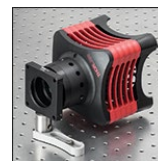
Click to Enlarge The SOLIS-1C shown mounted to an optical table using the SM2T2 adapter, a LCP01 60 mm cage plate, and a Ø1" post.
