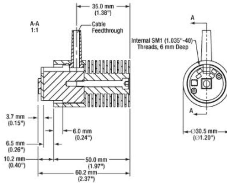
This LED features a Ø30.5 mm heat sink.
