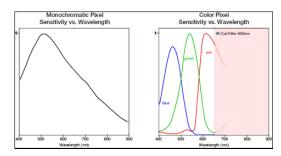
Due to this arrangement, each pixel is only sensitive to one color, and as a result,
