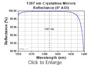
Click Here for Theoretical Data From 900 -1900 nm Theoretical Reflectance of 1397 nm Crystallin
