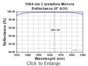
Click Here for Theoretical Data From 800 -1500 nm Theoretical Reflectance of 1064 nm Crystalline Supermirrors
