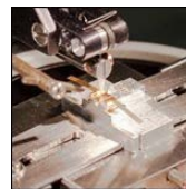
Click for Details Wire Bonding a Quantum Cascade Laser on a C-Mount
