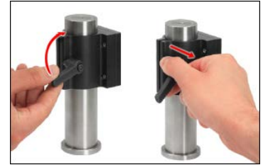
Click for Details Left: C15QR Quick-Release Handle Being Attached to the C1511 Post Mounting Clamp Right: Pull Back to Rotate the Position of the Handle
