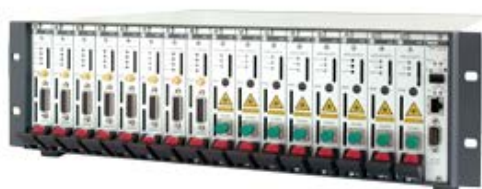
ITC5000 & LS5000 Modules in TXP5016 Chassis
