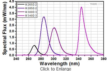
UV LED Spectra Scaled to Min Power
