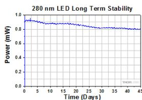
The M280L3 LED has a typical lifetime of  $>500$  hours. In this case, the unit under test has dropped to  $\sim 80\%$  of the initial output power after 45 days.
