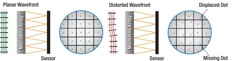
**Figure 1.** A planar wavefront incident on the Shack-Hartmann wavefront sensor's lenslet array and imaged on the CCD sensor will display a regularly spaced grid of spots. An aberrated wavefront, however, will cause individual spots to be displaced from the optical axis of each lenslet; if the displacement is large enough, the image spot may even appear to be missing. This information is used to calculate the shape of the wavefront that was incident on the microlens array.
