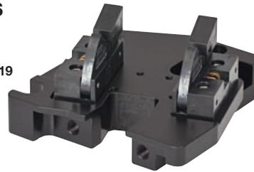
These half-butterfly gain chip mounts are designed to mount a 6-pin half-butterfly assembly in a Tunable Laser Kit. They angle the gain chip properly within the laser such that emitted light can be aligned to the external cavity. Half-butterfly mounts are available for 0°, 19.5°, and 26.5° exit angles. Please see the tables to the left to determine the exit angle of your gain chip.
