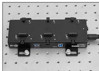
Click to Enlarge Figure 1.5 Each controller hub includes horizontal mounting brackets for securing the hub to an optical table or breadboard.
