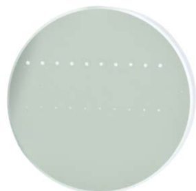
The photograph above is a protected aluminum-coated mirror after LIDT testing. In this particular test, it handled 0.43 \text{ J/cm}^2 (1064 nm, 10 ns pulse, 10 Hz, \text{Ø}1.000 \text{ mm} ) before damage.
