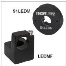
The LEDMF LED Mount is designed to hold any of Thorlabs' TO-18R packages directly or our T-1 3/4 or TO-18 packages using one of the included adapter rings (Ø4.7 mm adapter for TO-18 or Ø5 mm adapter for T-1 3/4). The LED is secured in the mount with a top-located cap screw with a 5/64" (2 mm) hex. The L-shaped mount has a counterbored through hole suitable for an 8-32 (M4) cap screw so that the LEDMF can be attached to a Ø1/2" Post.
