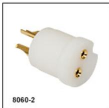
Thorlabs offers a light-emitting diode (LED) socket that is compatible with LEDs that have two leads. This socket fits LED leads that are Ø0.016" (Ø0.41 mm) and ≤0.22" (5.6 mm) long. The socket has gold-plated beryllium copper contacts and meets RoHS compliance.
