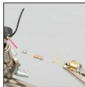
Find the positive pin on the LED, the anode, which can be found on the LED's Spec Sheet, and solder it to the resistor.
