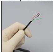
Strip the outer plastic about two inches from the end, being careful not to cut too far into the wire.
