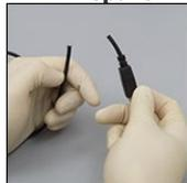
If the chosen USB wire is repurposed with two ends, unplug both ends and cut off the non-Type A Male end, leaving as much slack on the Type A Male end as possible using Wire Cutters.
