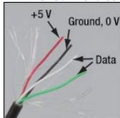
The wire will contain shielding and four smaller wires: Red (+5 V), Black (Ground, 0 V), White and Green. The latter two wires are used for data transfer.
