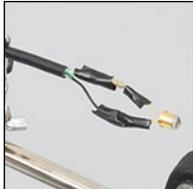
Once the solder has cooled, wrap each connection separately in a layer of electrical tape.
