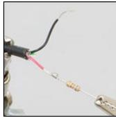
Solder one end of the resistor (resistors are bidirectional, either end will do) to the red wire. The end of the resistor's lead and the black wire should be roughly the same length.
