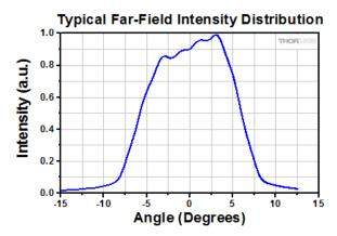
The typical far field intensity distribution is shown above, which was recorded 25 mm from the LED with the case temperature held at 25 °C. This data is for one particular diode; the performance will vary from device to device. To view an Excel file with raw data from the sample LED shown above, please click <a href="here">here</a>.
