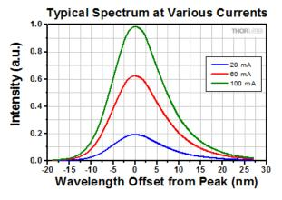
Typical spectra are shown above, all of which were obtained with the case temperature held at 25 °C.
