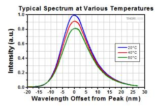
Typical spectra are shown above for a variety of temperatures, all of which were obtained with a pulsed driving current of 100 mA. This data is for one particular diode; the performance will vary from device to device. To view an Excel file with raw data from the sample LED shown above, please click <a href="https://pers.ncb//>
