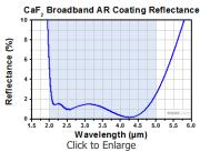
Click Here for an Excel File with Plot Data Shown above is a graph of the measured percent reflectance of the enhanced AR coating as a function of wavelength. The average reflectance in the 2 - 5 µm range is <1.25%. The blue shading indicates the region for which the AR coating is optnized. Performance outside of the specified range is not guaranteed and varies from lot to lot. The excel file above provides the coating curve data over an extended wavelength range.
