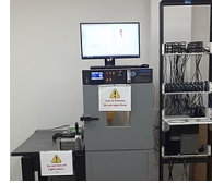
Click To Enlarge Damp Heat Testing Setup
