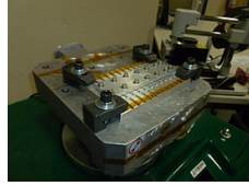
Click To Enlarge Close-Up of Mechanical Shock Test Setup
