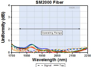
The plot above shows the uniformity measured at each output leg of four TW2000R3A2A couplers (tap and signal outputs from the same coupler indicated by matching colors). The blue-shaded region denotes the coupler's full operating wavelength range.
