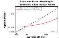
Wavelength (nm) Click to Enlarge Plot showing approximate input power that can be incident on a single mode silica optical fiber with a termination. Each line shows the estimated power level due to a specific damage mechanism. The maximum power handling is limited by the lowest power level from all relevant damage mechanisms (indicated by a solid line).
