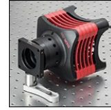
The SOLIS-1D shown mounted to an optical table using the SM2T2 adapter, a LCP34 60 mm cage plate, and a Ø1" post.
