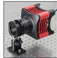
The SOLIS-1D shown mounted to an optical table using an SM2L15 lens tube, two SM2RC lens tube mounts, two Ø1/2" posts, and one BA2 post holder base.
