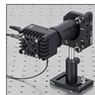
Click to Enlarge [APPLIST] [APPLIST] SA200-18C with PDA10PT Detector Installed
