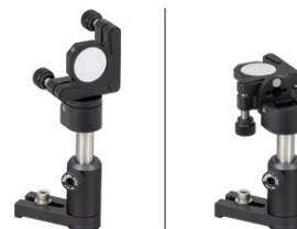
Click to Enlarge Figure 6: Flipper Mirror in the Up Position (left) Intercepts Beam and Directs it to Interferometer Setup. Flipper Mirror in the Down Position (right) Allows Beam to Downstream Optics.
