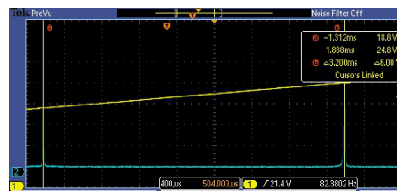
Figure 1: An FSR Plot, Using a 1550 nm DFB Laser (PRO8000 Series). Using the SA200-12B
