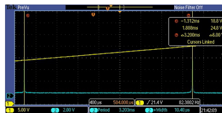
Figure 1: An FSR Plot, Using a 1550 nm DFB Laser (PRO8000 Series). Using the SA200-12B
