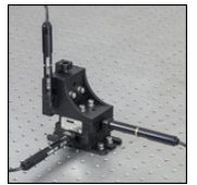
Click to Enlarge Three MT1-Z8 Single-Axis Stages Mounted into an XYZ Configuration via an MT402 Right-Angle Bracket
