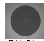
Click to Enlarge Undamaged Fiber End
