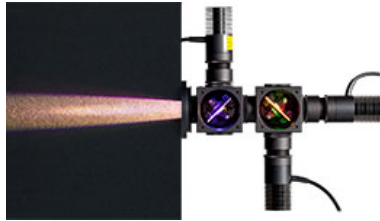
Beam Profile of Source with 3 Mounted LEDs
