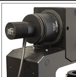
The MWWHL4 LED and COP1-A microscope collimation adapter used as a trans-illumination source for an Olympus microscope.
