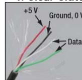
The wire will contain shielding and four smaller wires: Red (+5 V), Black (Ground, 0
