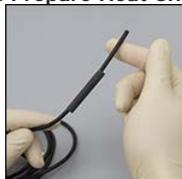
If heat shrink tubing will be utilized, place a length of two inches down the wire
