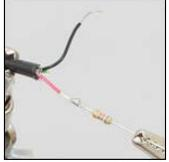
Solder one end of the resistor (resistors are bidirectional, either end will do) to the red wire. The end of the resistor's lead and the black wire should be roughly the same length.
