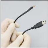
Either cover the wrapped wires in electrical tape, or, if heat shrink tubing was placed down the wire, slide it up over the connections, and slowly heat with a heat gun or hair dryer until it snugly fits over the connections.
