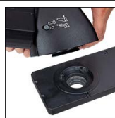
Click to Enlarge This photo shows the male D1N dovetail on the trinoculars next to the female D1N dovetail on the epi-illumination arm.
