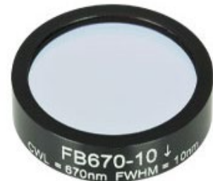
FB670-10 Ø1" Filter CWL = 670 nm, FWHM = 10 nm
