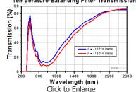
Click to Download an Excel File of Raw Data The graph above shows the measured transmission curve for a filter with a conversion value (V) of -132 mireds and a filter with a conversion value of -160 mireds. For details on the mireds unit, please see the
