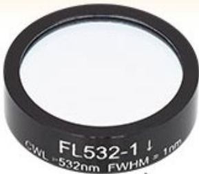
FL532-1 Ø1" Filter CLW = 532 nm, FWHM = 1 nm
