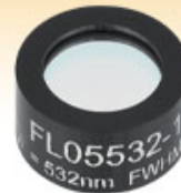
FL05532-1 Ø1/2" Filter CWL = 532 nm, FWHM = 1 nm
