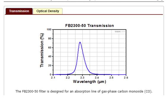
FB2300-50 - Ø25 mm IR Bandpass Filter, CWL = 2.30 µm, FWHM = 50 nm
