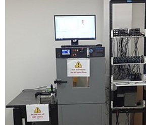
Click To Enlarge Damp Heat Testing Setup
