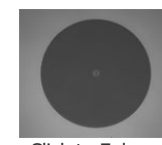
Click to Enlarge Undamaged Fiber End
