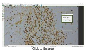
**Figure 2:** A screenshot of the ThorCam software showing some of the analysis and annotation features. The Tally function was used to mark four locations in the image. A blue crosshair target is enabled and locked to the center of the image to provide a point of reference.
