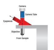
When viewing an image with a camera, the system magnification is the product of the objective and camera tube magnifications. When viewing an image with trinoculars, the system magnification is the product of the objective and eyepiece magnifications.
