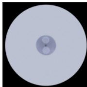
Click to Enlarge View of PANDA-Style PM Fiber with the FS201 Inspection Scope and FS201-PM Adapter
