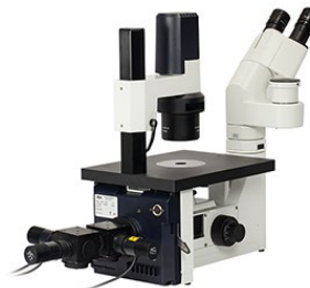
Click to Enlarge Multi-LED Source Coupled to Microscope Illumination Port
