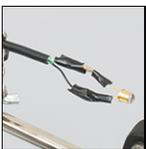
Once the solder has cooled, wrap each connection separately in a layer of electrical tape. Warning: Improper insulation of exposed metal can lead to shorting of the circuit, electrical failure, or fire.
