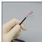
Strip the outer plastic about two inches from the end, being careful not to cut too far into the wire.
