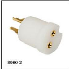
Thorlabs offers a light-emitting diode (LED) socket that is compatible with LEDs that have two leads. This socket fits LED leads that are Ø0.016" (Ø0.41 mm) and ≤0.22" (5.6 mm) long. The socket has gold-plated beryllium copper contacts and meets RoHS compliance. Color varies by lot and may be white, off white, black, or tan.
