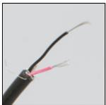
Cut away an inch of the red wire, any exposed shielding, and the white and green wires down to the main wire's remaining outer plastic while stripping the Red and Black wires to give enough room for a solder joint.
