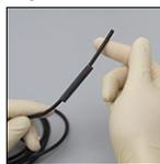
If heat shrink tubing will be utilized, place a length of two inches down the wire for later.
