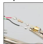
Solder the remaining, negative end of the LED, the cathode, to the black wire.
