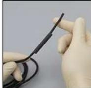
If heat shrink tubing will be utilized, place a length of two inches down the wire for later.
