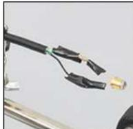
Once the solder has cooled, wrap each connection separately in a layer of electrical tape.
