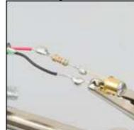
Solder the remaining, negative end of the LED, the cathode, to the black wire.
