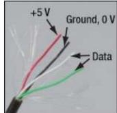
The wire will contain shielding and four smaller wires: Red (+5 V), Black (Ground, 0 V), White and Green. The latter two wires are used for data transfer.
