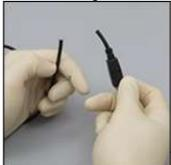
If the chosen USB wire is repurposed with two ends, unplug both ends and cut off the non-Type A Male end, leaving as much slack on the Type A Male end as possible using Wire Cutters.
