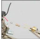
Find the positive pin on the LED, the anode, which can be found on the LED's Spec Sheet, and solder it to the resistor.
