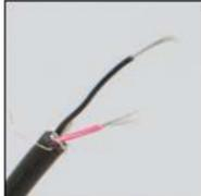
Cut away an inch of the red wire, any exposed shielding, and the white and green wires down to the main wire's remaining outer plastic while stripping the Red and Black wires to give enough room for a solder joint.
