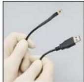
Either cover the wrapped wires in electrical tape, or, if heat shrink tubing was placed down the wire, slide it up over the connections, and slowly heat with a heat gun or hair dryer until it snugly fits over the connections.
