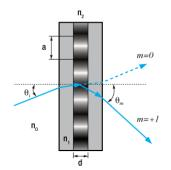
Figure 8. Volume Phase Holographic Grating
