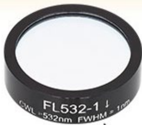
FL532-1 Ø1" Filter CLW = 532 nm, FWHM = 1 nm
